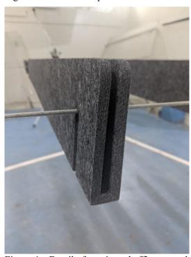
Figure 4 – Detail of specimen baffle suspended from cables using notches
